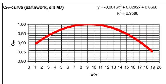
fig.1. Curve of moisture correction coefficient
