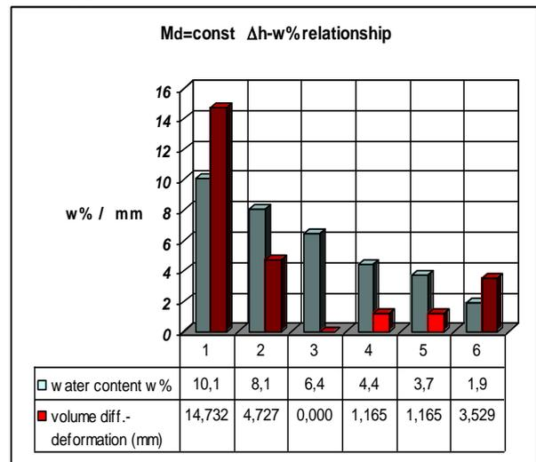
fig.2 Height difference of Proctor-rolls ( $M_d$ =constant)
