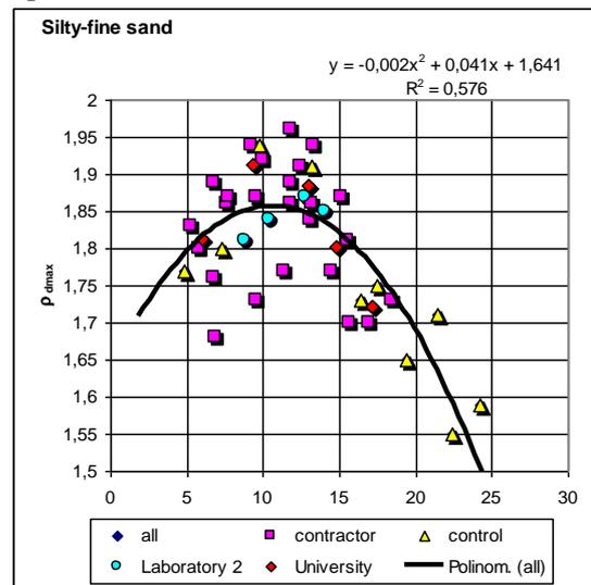
fig.4 Proctor-points one sample – four laboratory
