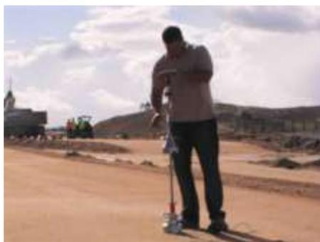
Picture 7-8. B&C ANDREAS new dynamic compactness and bearing capacity measuring device
