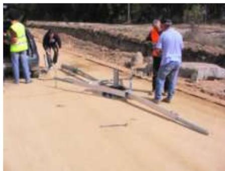
Pictures 16-17. Static load bearing capacity test with D=600mm plate
