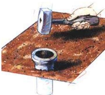
Picture 12. Tube sampling method
