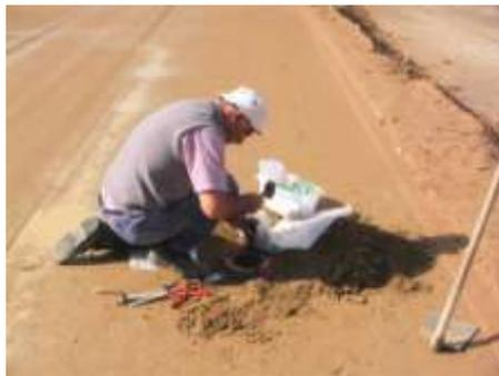
Pictures 5-6. ASTM Sand-filling test
