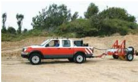
Pictures 10-11. Portancemetre continuous load bearing capacity measuring method
