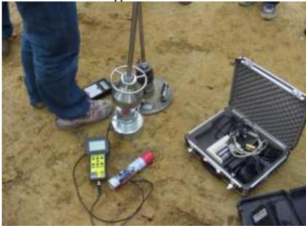
Picture 9. Small plate and Big-plate LFWD light falling weight devices
