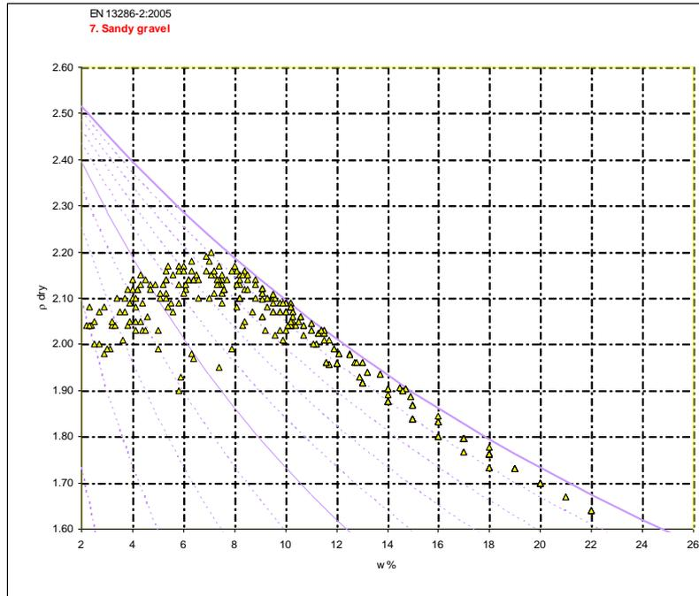
Figure 2 Proctor round test: sandy Gravel (saGr)
