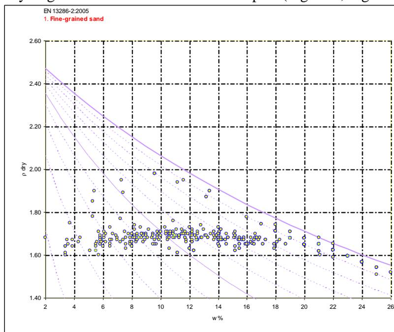
Figure 1 Proctor round test: Fine-grained sand (siSa)
