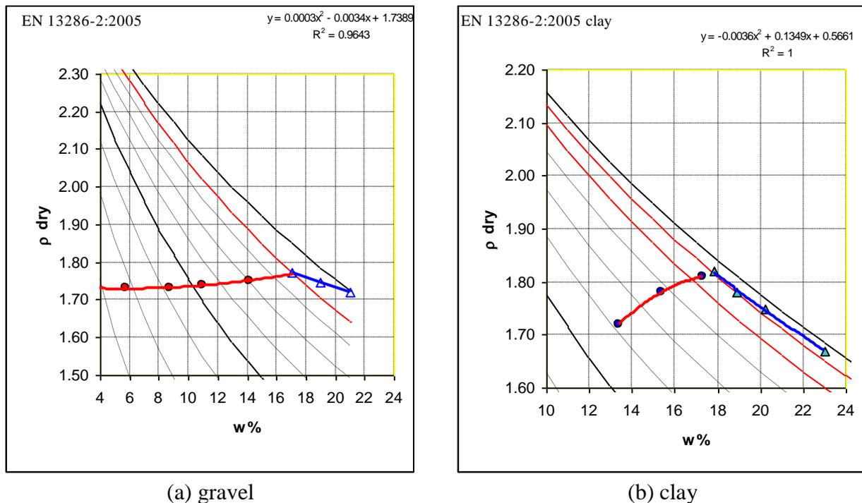
Figure 4 Proctor curve processed with the new two-branch method
