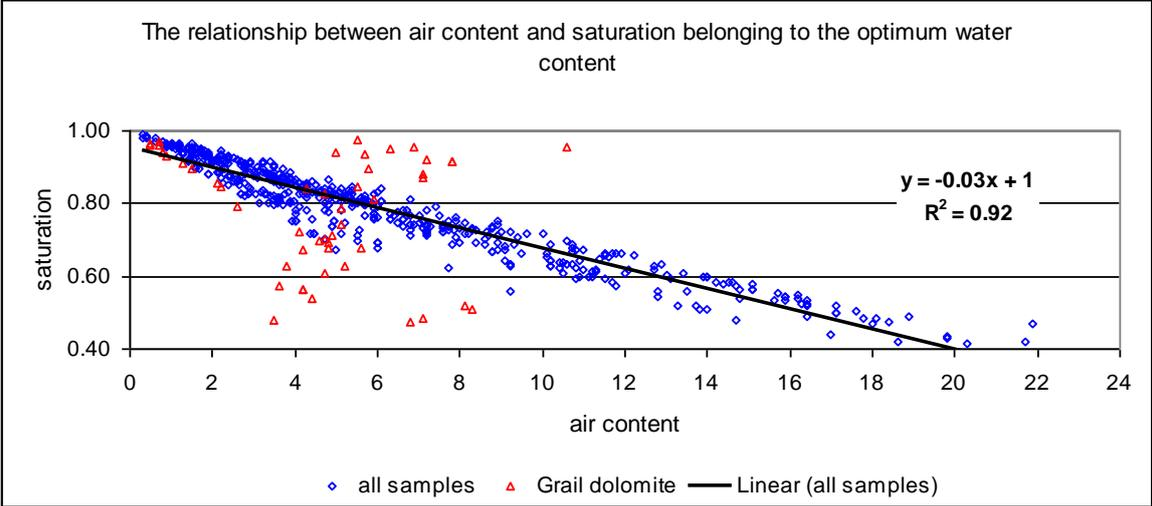
Figure 10 General relationships between the air content and the saturation belonging to  $w_{opt}$
