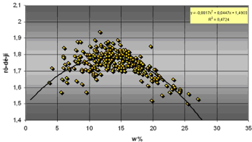
Figure 3 Proctor points measured by different accredited laboratories from one soil sample
