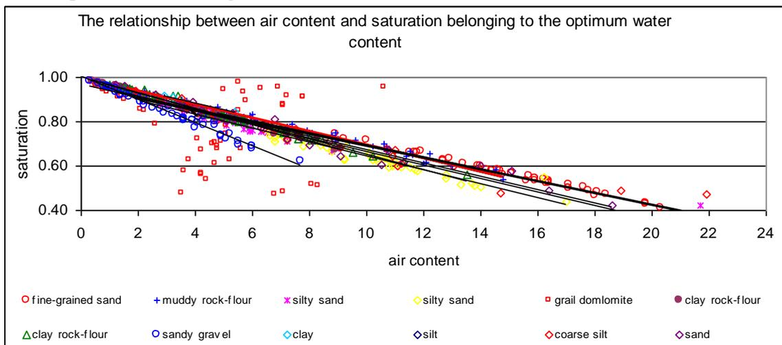
Figure 9 Relationship between the air content and the saturation belonging to  $w_{opt}$
